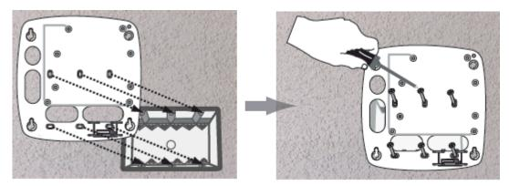
3. Pull the wires from the gang box through the knockout holes in the base of the enclosure.
